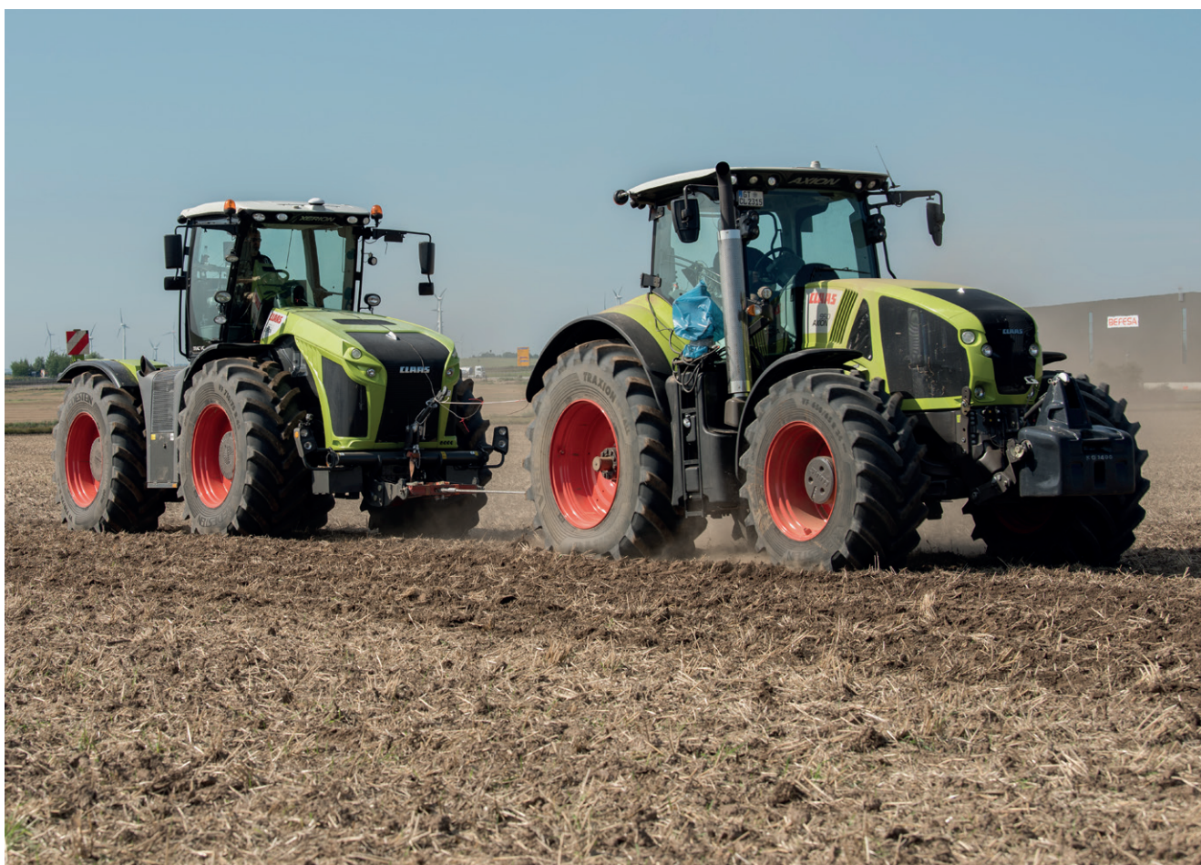
Figure 2: Towing tractor and braking tractor in use
